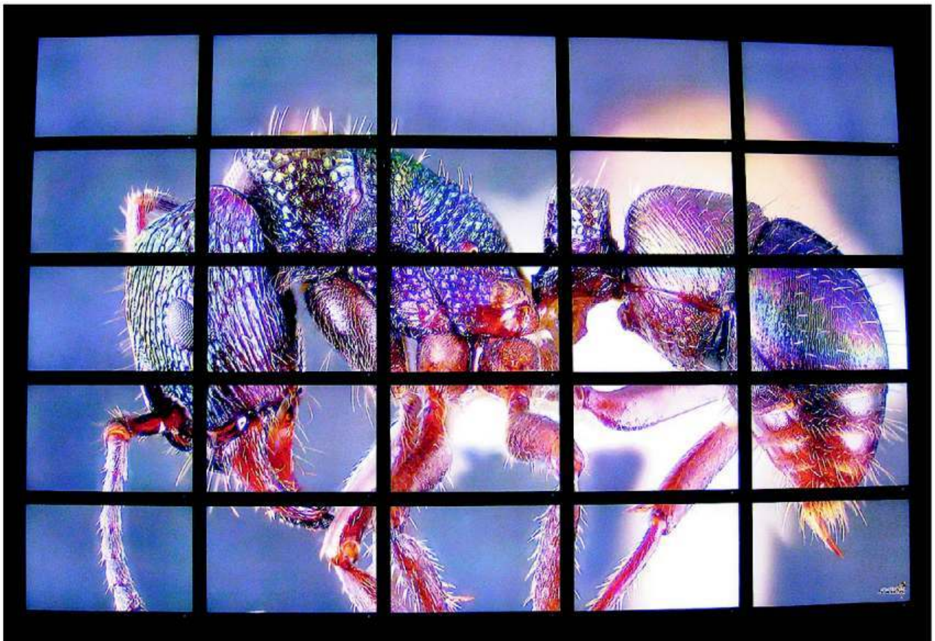
CRYSTAL CLEAR: A close-up of an ant on the CSIROvision’s array of five by five LCD screens. The visualisation system can display video, data and images. Photo: CSIRO
